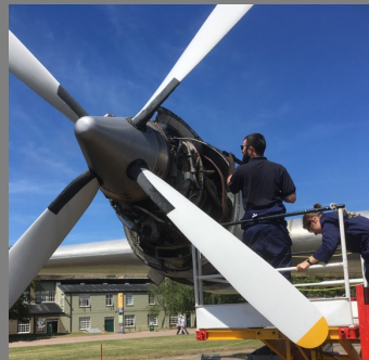
Ongoing maintenance on the large turboprop engine Photo: Chrissie Eaves-Walton
